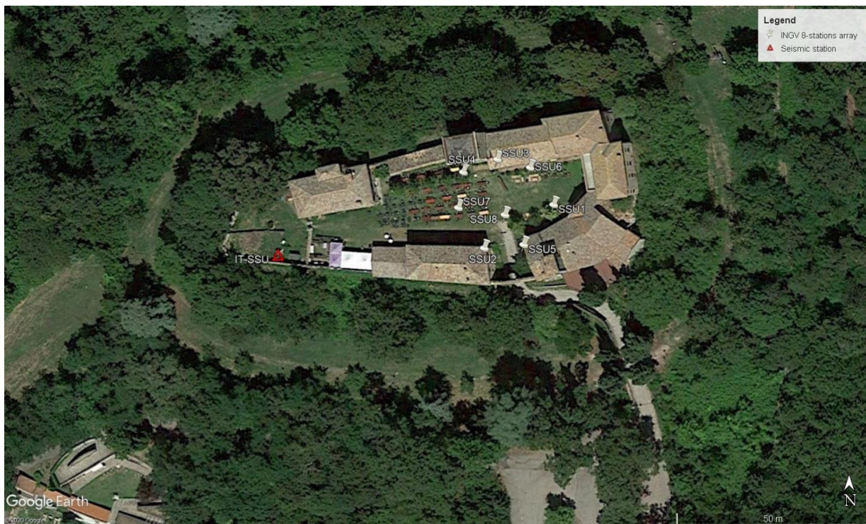
Figure 6: Map of the geophysical measurements performed at the IT.SSU site. The white placemarkers in circular geometry are the 8 stations of the 2D array in passive configuration. The red triangle indicates the IT.SSU accelerometric station (image from Google Earth http://www.earth.google.com ).
