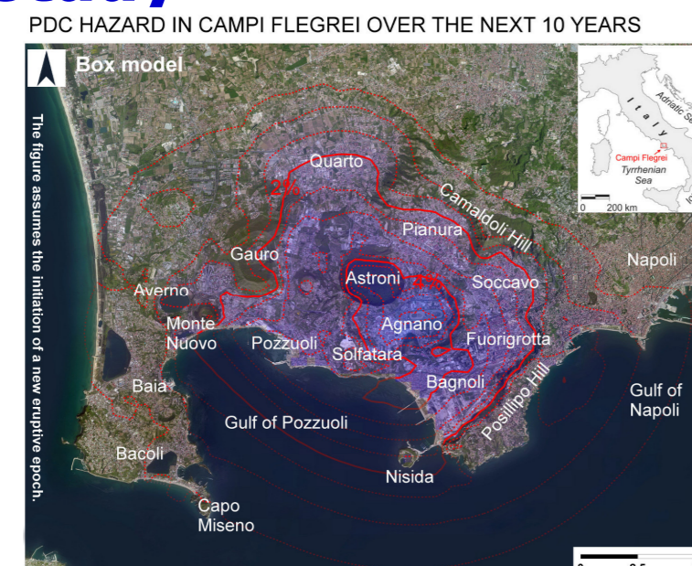
Figure 2. Example of temporal PDC invasion hazard map based on Bevilacqua et al. (2017), assuming that the volcano entered a new eruptive epoch in A.D. 1538. Contours and colors indicate the mean percentage probability of PDC invasion in the next 10 years.
