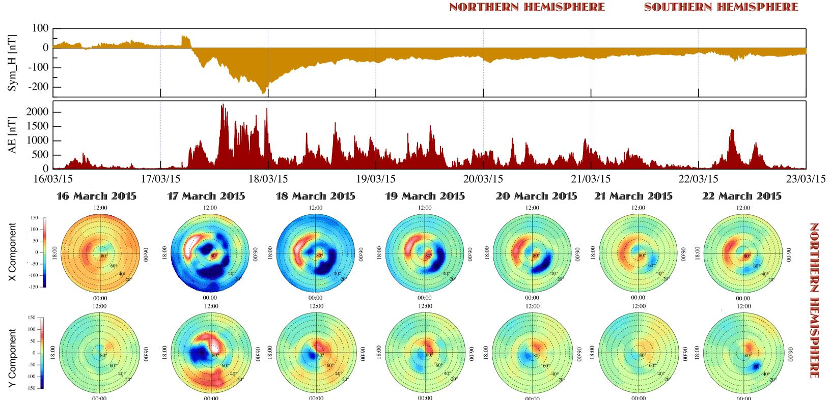
Daily distributions of the X and Y magnetic field components. Maps describe the magnetic field perturbations on the ground due to external sources. The main contributions to this external fields, that produce relevant signatures in magnetic field observations, are the polar ionospheric currents, such as the polar electrojets, and the magnetospheric currents such as the Chapman-Ferraro currents and in particular the ring current.
