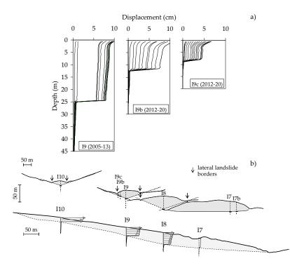
**Figure 4.** *Costa della Gaveta* earthflow: inclinometer profiles I9, I9b, and I9c (**a**); longitudinal section with inclinometer profiles relative to the same time period and transversal sections (**b**).
