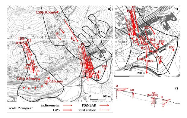
**Figure 14.** Vectors of average rates of horizontal displacements obtained from inclinometer, GPS, and PSInSAR data in the period May 2011–March 2014 and from topographic measurements carried out in 2010–2011 (**a**); zoom (**b**) and longitudinal section (**c**) of *Varco d'Izzo* earthflow accumulation.
