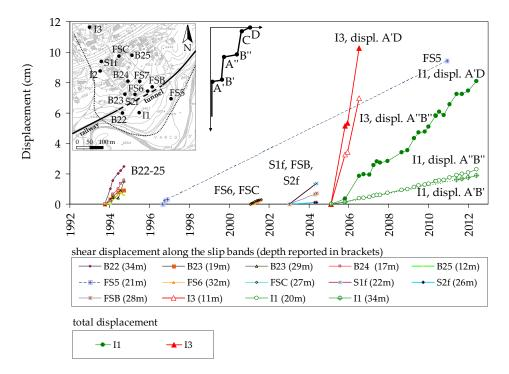
**Figure 7.** Deep and total displacements in different areas of the *Varco d'Izzo* earthflow, obtained from inclinometer data (redrawn from Di Maio et al. [42]).
