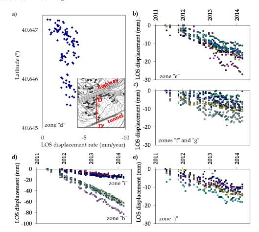
**Figure 13.** (a) LOS displacement rate against latitude along DD'; (**b**–**e**) LOS displacement time series of the groups of scatterers "e"–"j" (location in Figure 11).
