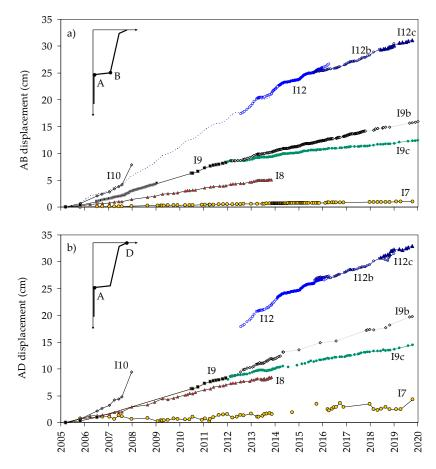
**Figure 5.** Time series of cumulative deep displacements AB (**a**) and superficial displacements AD (**b**) of *Costa della Gaveta* landslide, obtained from inclinometer data.
