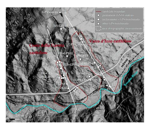
**Figure 2.** *Costa della Gaveta* and *Varco d'Izzo* earthflows and location of inclinometers, GPS stations and benchmarks, and area of topographic measurements.
