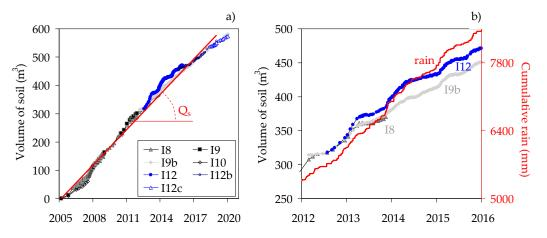
**Figure 15.** *Costa della Gaveta* earthflow: volumes of soils, with an indication of the average soil discharge Q<sub>s</sub>, crossing the transverse sections through the inclinometers (**a**), and comparison with cumulative rain (**b**).
