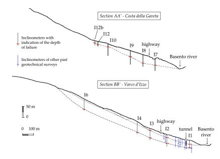
**Figure 3.** Sections AA' and BB' with inclinometers of recent and past surveys, depth of failures, and hypothesized slip surfaces.
