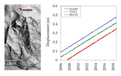
**Figure 8.** Displacement time series in the IGS14 coordinate system of the master station and two other permanent stations located in the same sector of the Southern Italian Apennines: MATE (operated by ASI—Italian Space Agency) and TITO (operated by CNR—National Research Council of Italy).
