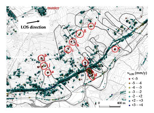
**Figure 11.** Average rates of the line of sight (LOS) displacement of monitored scatterers in the period May 2011–March 2014 evaluated from COSMO-SkyMed ascending data.
