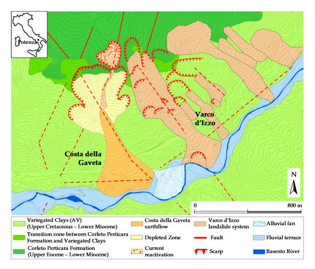
**Figure 1.** Geological map of the *Costa della Gaveta* earthflow (redrawn from [24]), and the *Varco d'Izzo* landslide system (redrawn from [26]).
