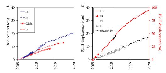
**Figure 9.** Comparison of: inclinometer and GPS data of *Costa della Gaveta* earthflow (**a**); inclinometer, GPS, and theodolite data of *Varco d'Izzo* earthflow (**b**).
