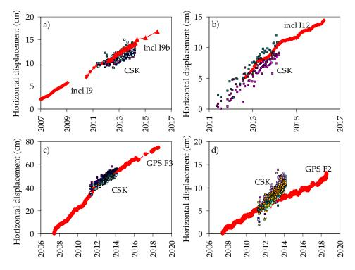
**Figure 12.** Comparison of displacements obtained from PSInSAR data, GPS, and inclinometers in zones (a), (b), (c), and (d) of Figure 11.
