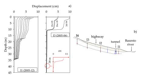
**Figure 6.** Inclinometer profiles I1 and I3 (**a**) and longitudinal section of the lower *Varco d'Izzo* earthflow (**b**). I3 went out of use in a year along the shallower slip surface, when the displacements on the deeper slip surface were small (as visible in the zoom relative to the profile of December 2005).
