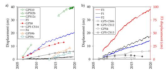
**Figure 10.** Displacements of GPS stations and benchmarks of *Costa della Gaveta* (**a**) and *Varco d'Izzo* (**b**) earthflows.
