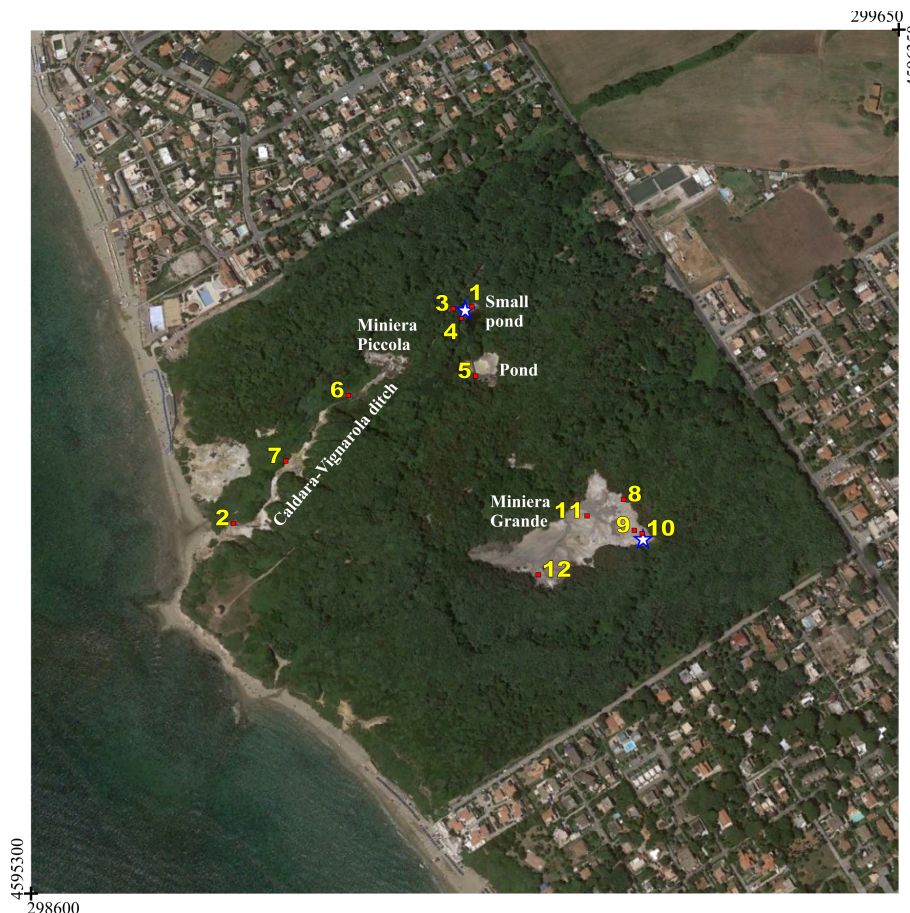
Figure 1. Tor Caldara natural reserve with the location of the main gas discharge zones (Miniera Grande, Miniera Piccola, ponds and Caldara-Vignarola ditch). The yellow numbers and red dots indicate the sites where air gas concentration has been continuously monitored in March-July 2012. The two white stars indicate the location of the meteo-station.
