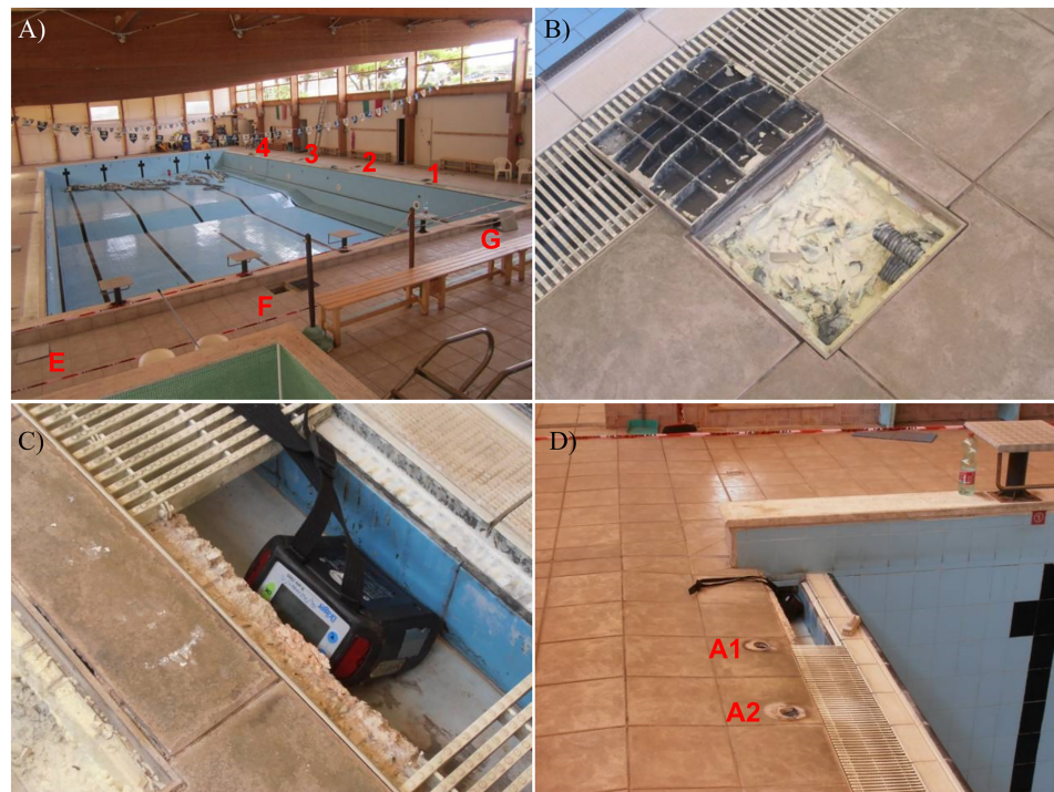
Figure 10. (a) The Lavinio Country Club swimming pool with the location of 1 to 4 light housings. (b) Light housing no. 1 with sulfur incrustations. (c) Device measuring gas air concentration placed into a lateral overflow channel. (d) Stair-anchoring bores no. A1 and A2 and the nearby overflow channel. See Figure 3 for the precise location of these sites.
