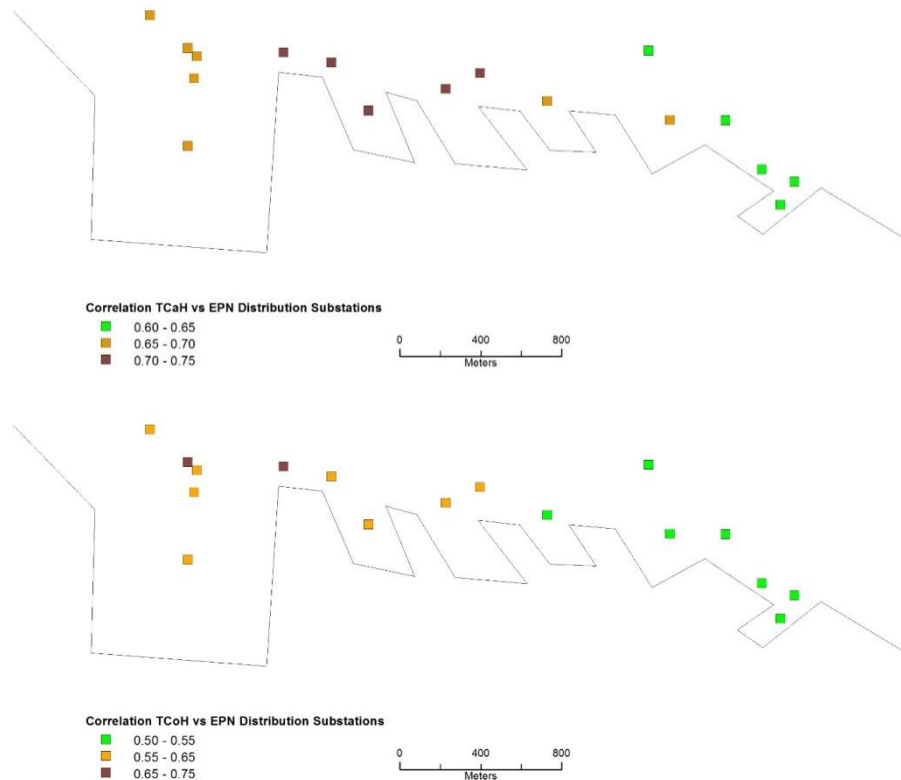
Figure 16. Correlation of non-functional EPN distribution substations to port performance (TCaH and TCoH) for ST-L2 due to ground shaking
