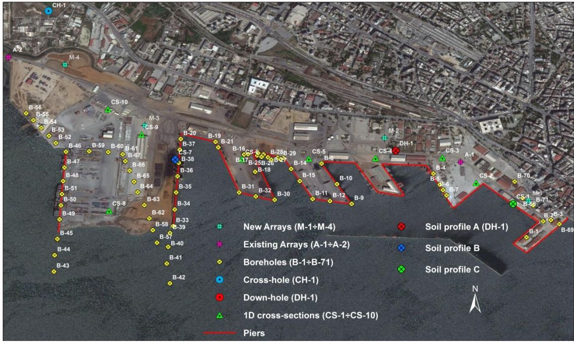
Figure 3. Location of geotechnical tests and geophysical field measurements in Thessaloniki's port area
