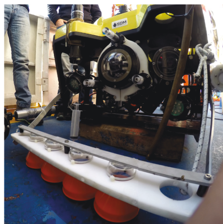
FIGURE 3: Sampling system for the bubbling gases off Zannone (depth in the range of 120-150 m bsl). The ROV was equipped with a homemade sampling system composed of four small funnels connected to 240 ml serum-type bottles. The system, fitted to the front of the ROV, allows to collect bubbles by placing the funnel on the venting gases (see text for more information).
