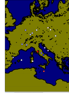
Fig. 3: Directivity analysis shows a clear pattern of variations of the apparent durations with azimuth, although the event is of moderate magnitude (M4.5), indicating a bilateral rupture, along the dip in direction NNE-SSW, rather than along the strike.
