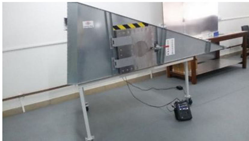
Figure 11. Scaled down bent wire dipole antenna characterisation in GTEM cell setup
