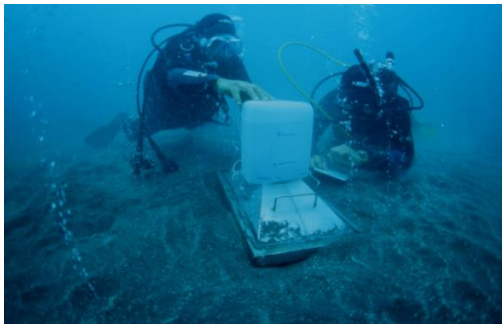
Figure 2 Gas output measurement performed by scuba-divers (ranging around 107 liters per day during quiet periods).
