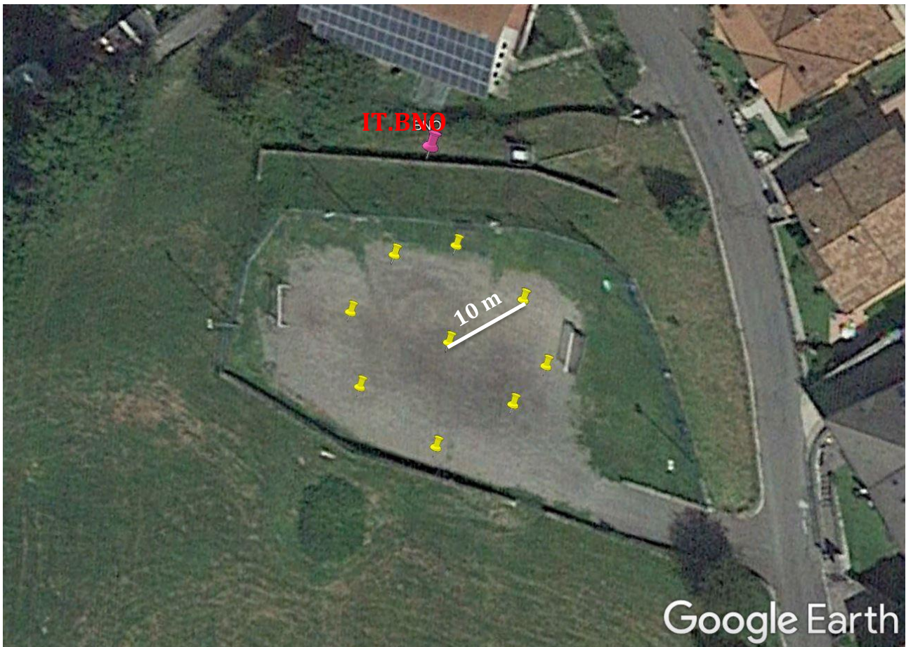
Figure 1: Map of the geophysical measurements performed at the IT.BNO site. The yellow points are the nine stations of the 2D array in passive configuration. The red point indicates the IT.BNO seismic station.
