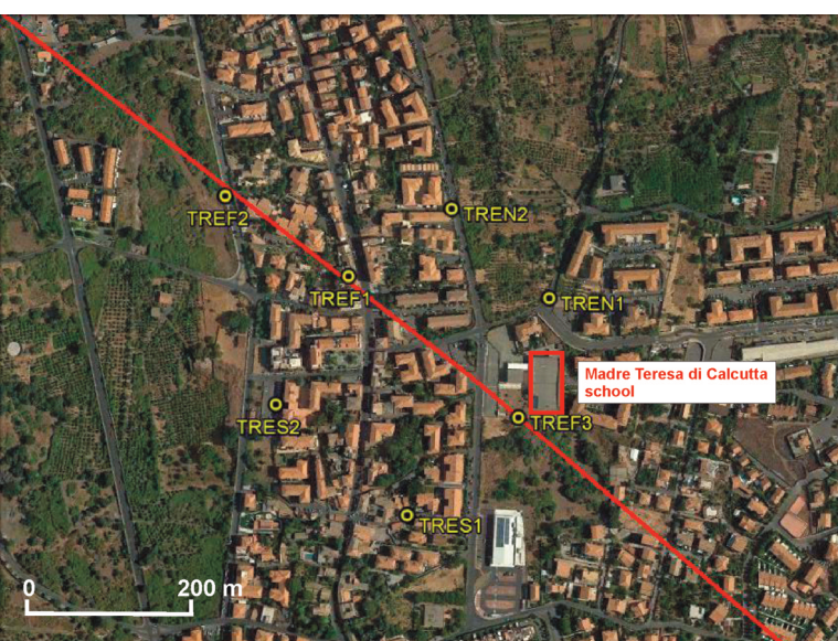
FIGURE 2. Localization of mobile seismic stations and the Madre Teresa di Calcutta school. Red line indicates the fault trace identified by surface evidence.
