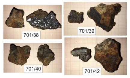
Figure 2. Studied iron slag samples characterized by the pseudo spherical shape, spongy appearance and rust color. Sample 701-38 shows the presence of vacuoles filled by secondary carbonate deposition.
