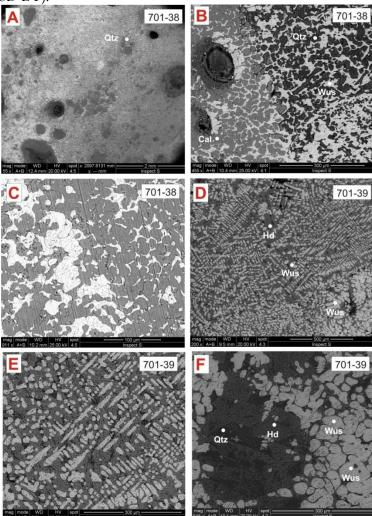
Figure 3. ESEM-EDX images showing textural features of slag samples 701-38 and 701-39. Qtz: Quartz; Cal: Calcite; Wus: Wustite; Hd: Hedembergite
