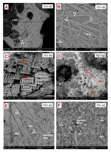
Figure 4. ESEM-EDX images showing textural features of slag samples 701-40 and 701-42. Qtz: Quartz; Fa: Fayalite; Wus: Wustite; Hd: Hedembergite
