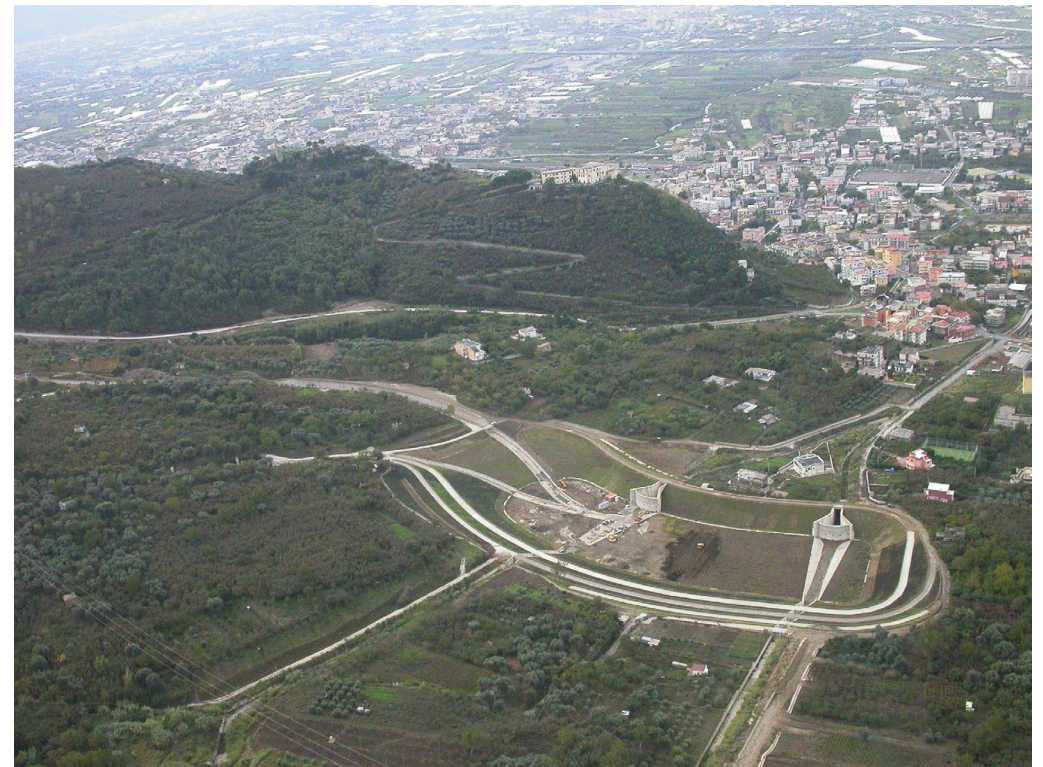
Fig. 17 - Engineering works built after the 1998 landslides at Sarno. In the foreground, Episcopio retention basin (net capacity: 176,000 m 3 ), designed to collect water and debris coming from the Trave, San Chirico, Cantariello and Licinatonda sub-basins.
