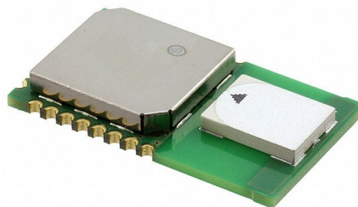
Figure 3. Ultra wideband (UWB) module: Decawave Sensor DWM1000.
