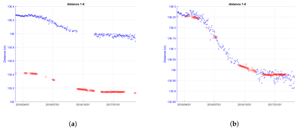
Figure 9. Comparison between the Wi-GIM UWB (blue crosses) and the RTS (red circles) systems to measure the distance between node 1 and 6 (Cluster 1—Roncovetro). (a) Data averaged over one day without offset compensation; (b) Data averaged over one day with offset compensation.
