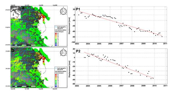
Figure 7. Augusta Bay subsidence revealed by C-band ENVISAT ascending (a) and descending (b) data.
