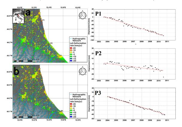
**Figure 3.** Deformation trend of Ravenna coastal area retrieved by ascending (**a**) and descending (**b**) ENVISAT data. On the right panels, the time series extracted by three points on the two maps are shown.
