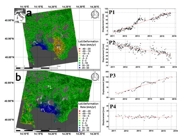
**Figure 5.** Campi Flegrei 2011–2015 uplift highlighted by COSMO-SkyMed interferometric synthetic aperture radar (InSAR) data. Deformation trend estimated along the ascending (**a**) and descending (**b**) orbits. In the right panels, the time series of four points are shown.
