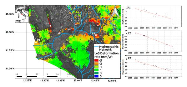
**Figure 4.** Deformation trend and time series for the Fiumicino area. These outcomes were retrieved by a dataset of 38 C-band ENVISAT images.
