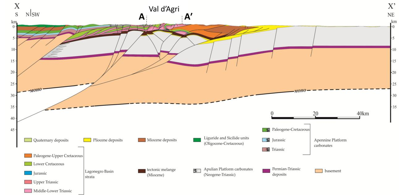
Crustal geological section (after Mazzoli et al., 2013, modified; Santini et al., 2013). The AA' cross-section through the Basilicata oil fields of Alta Val d'Agri has been constructed by the interpretation of available high-quality seismic data (Shiner et al., 2004).
