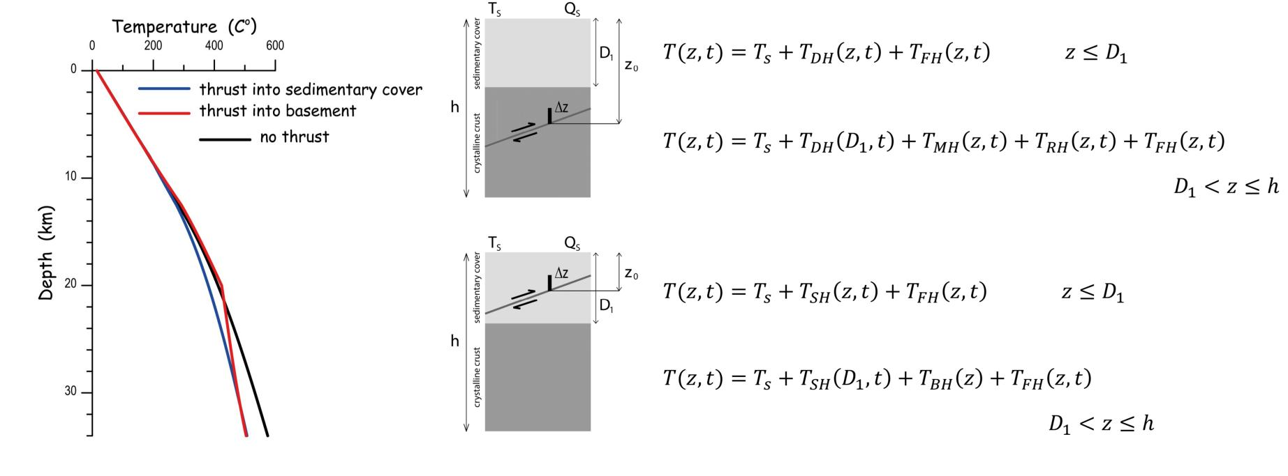
The consequences of overthrusting are a different distribution of the temperature due to new perturbed state and an increase of temperature due to friction.
