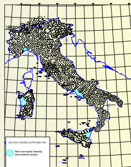
Italian II order network undertaken by CNR-PFG for elements F, H and Z: the measurements have been made in years 1977-1981
