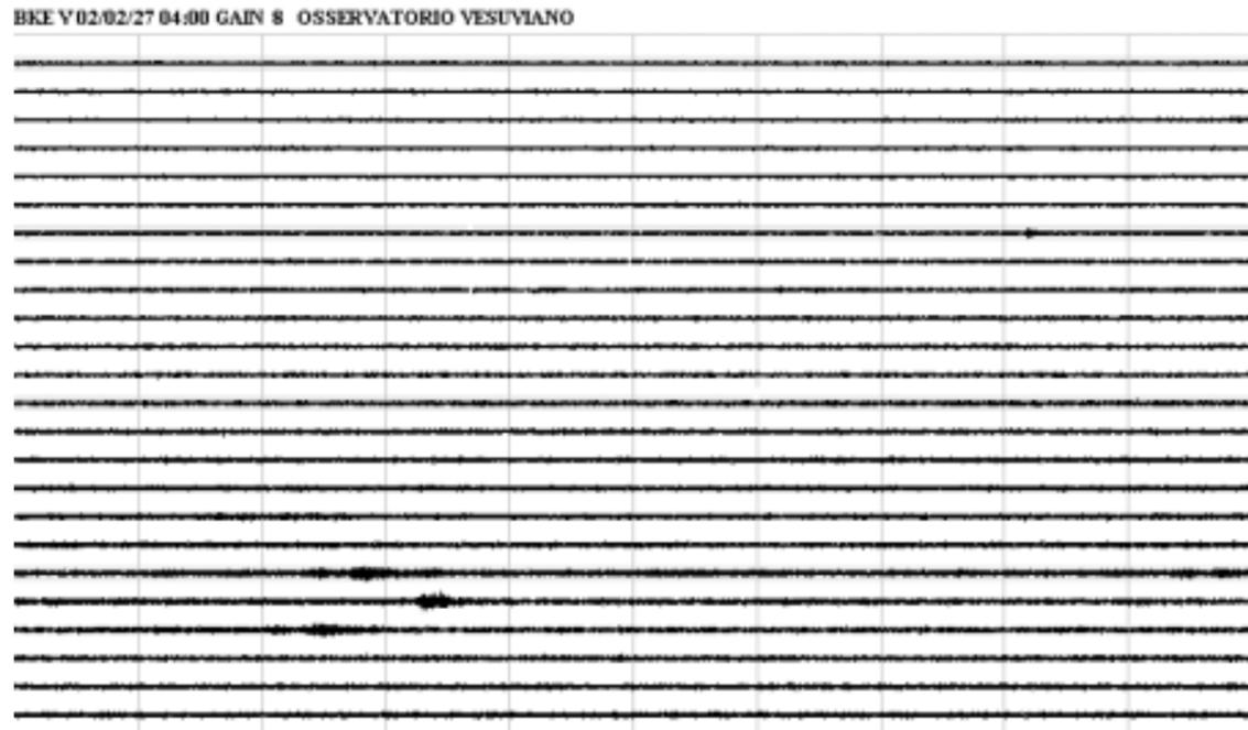
**Figure 4.** Seismic signal of BKE station (vertical component) starting at 04:00 to 08:00 U.T. (each line is ten minutes). Can be noted the increase of the noise amplitude due to cultural activity in the early hours of the morning.
