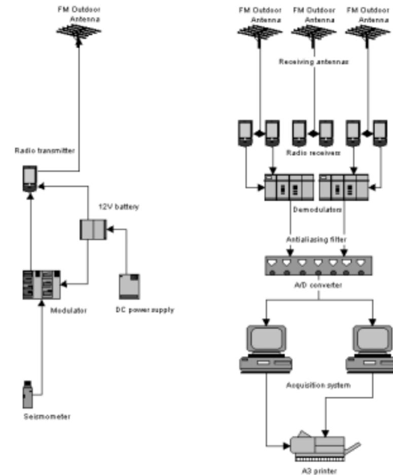
**Figure 3.** Block diagram of a typical telemetered analog short period seismic station and the Acquisition system.
