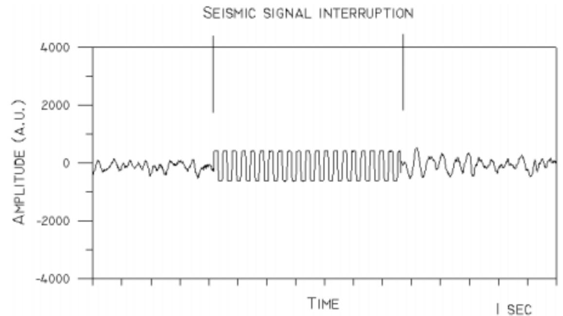
**Figure 8. b)** Example of control signal on phone line in case of seismic modulator failure. A 3 Hz square wave is broadcast with the same carrier frequency of the seismic signal [from Buonocunto 2002, modified].
