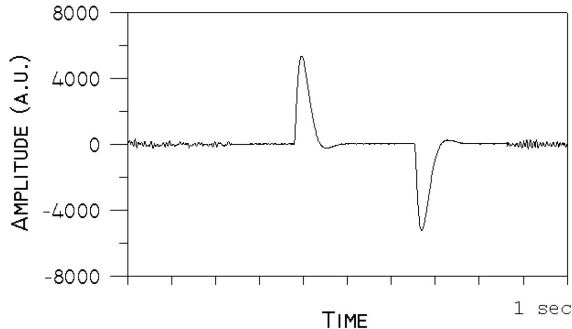
**Figure 7.** Daily calibration pulse at the CPV station. Calibration signal is short as possible to minimize the seismic signal interruption. The circuit provides to change the amplification to unitary value before the pulse, and it restores the operative amplification after the pulse.
