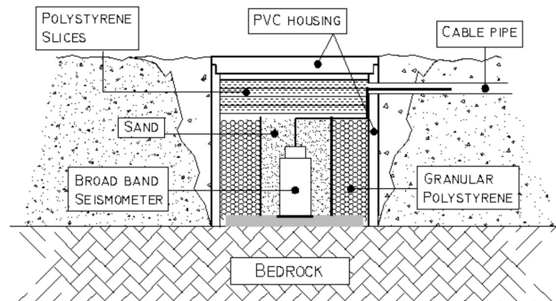
**Figure 6.** Detail of a broad band seismometer installation. Several level of insulation are used to keep stable the temperature.
