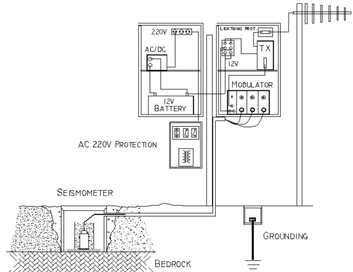
**Figure 5.** Scheme of a free field installation. Seismometer installation in a vault on bedrock is shown. The datalogger (modulator in this case) installation is also shown as described in chapter 6. AC protections comprise an insulating 220V AC line transformer, a lightning protector and circuit breakers for both magnetothermal and differential protection. Dimension of the single elements (seismic vault, equipment, AC protection, grounding, antenna) are not in scale.
