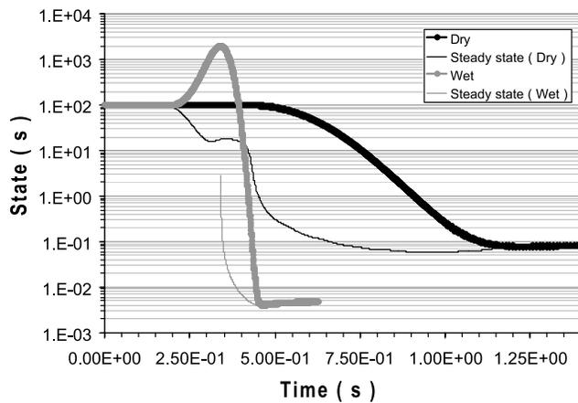
**Figure 10.** State variable evolution for the configurations showed in Figure 9. Black curves refer to dry faults, while grey ones to wet faults. Solid curves are the results of the numerical experiments, and thin lines represent the steady state value ( $\Psi^{ss}$ ) of the state variable.
