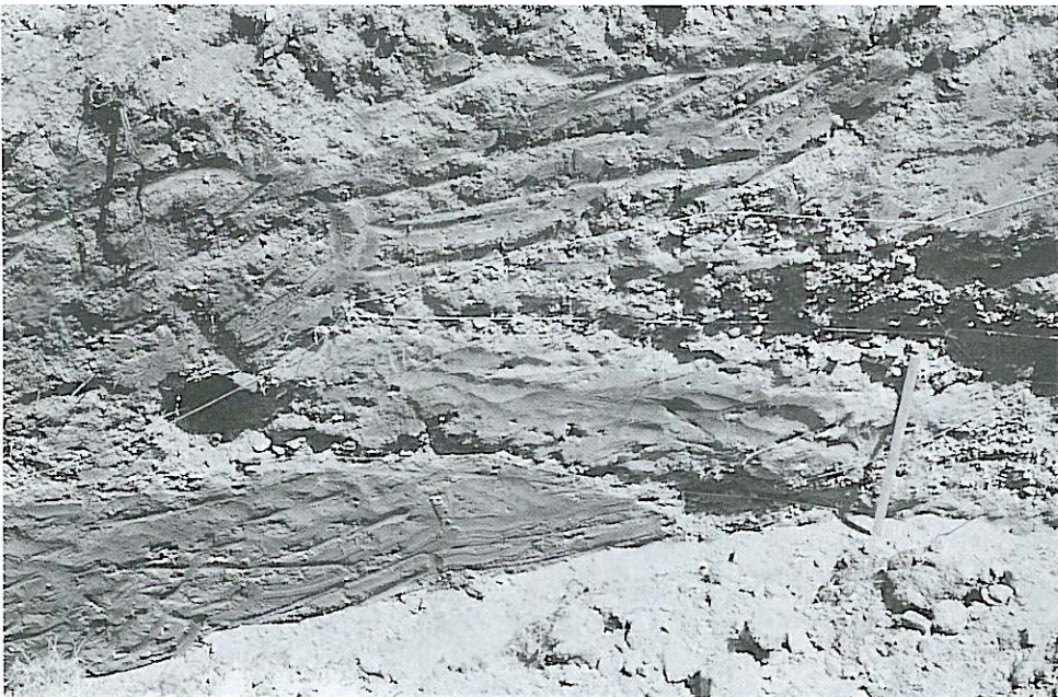
Fig. 11. View on the eastern wall of trench 3 (fig. 7). Structures suggest reverse faulting.
