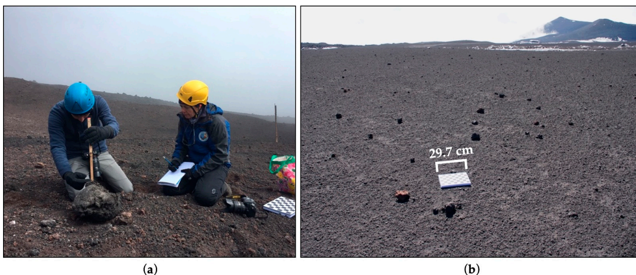
Figure 3. The sampling campaign was carried out on the southern side of Etna, at an altitude between 2600 and 2800 m a.s.l. (a) Measurements of one of the principal axes of a decimetric bomb. (b) Ballistics found on the ground level at about 2700 m.
