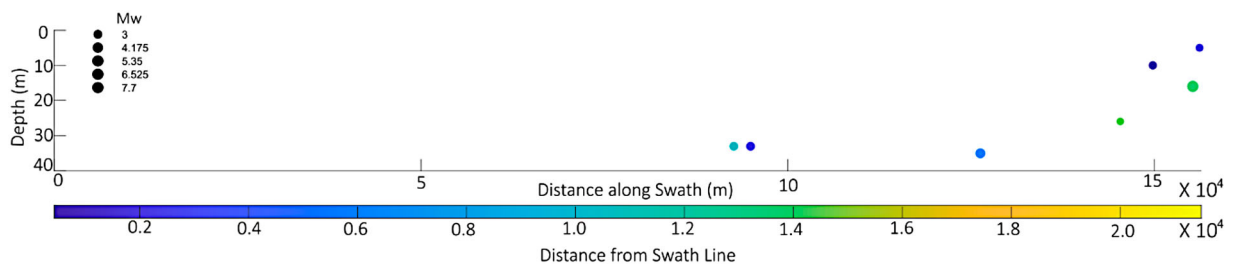
Figure 7. Swath-section, along the X-X' swath profile shown in Fig. 5, depicting the hypocenters from the revised literature. Circles represent the hypocenters of seismic events in the Kachchh Basin collected in a 40 km width swath and plotted along the cross-section. The colour code represents the distance from the swath baseline, and the circle's size represents the event's magnitude.
