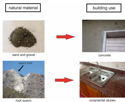
FIGURE 6. Natural materials are extensively used in construction. For instances, sands and gravel are used to produce concrete, whereas rocks are mined and used as ornamental and pavement stones. If rocks and sediments contain a large amount of radionuclides and they are used to create building components, then, their occurrence in walls, floor and furniture could be dangerous.
