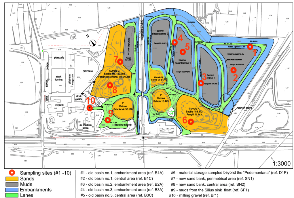
Figure 2. The Assemini waste area. The red circles are the sampling sites, with related labels and description, modified after [25].
