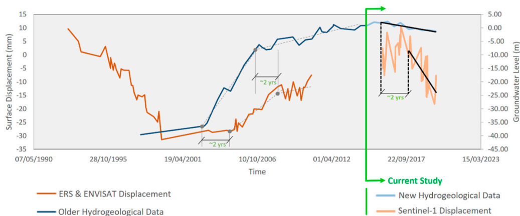
Figure 8. PSI based surface displacement vs. in-situ underground water level. Older data, corresponding to the period 1990–2014, were derived from the interferometric processing of ERS and ENVISAT data as well as in-situ water level measurements as reported in [14]. Whenever there is a trend change in the underground water level, surface deformation follows this change with an approximate time-lag of two years.
