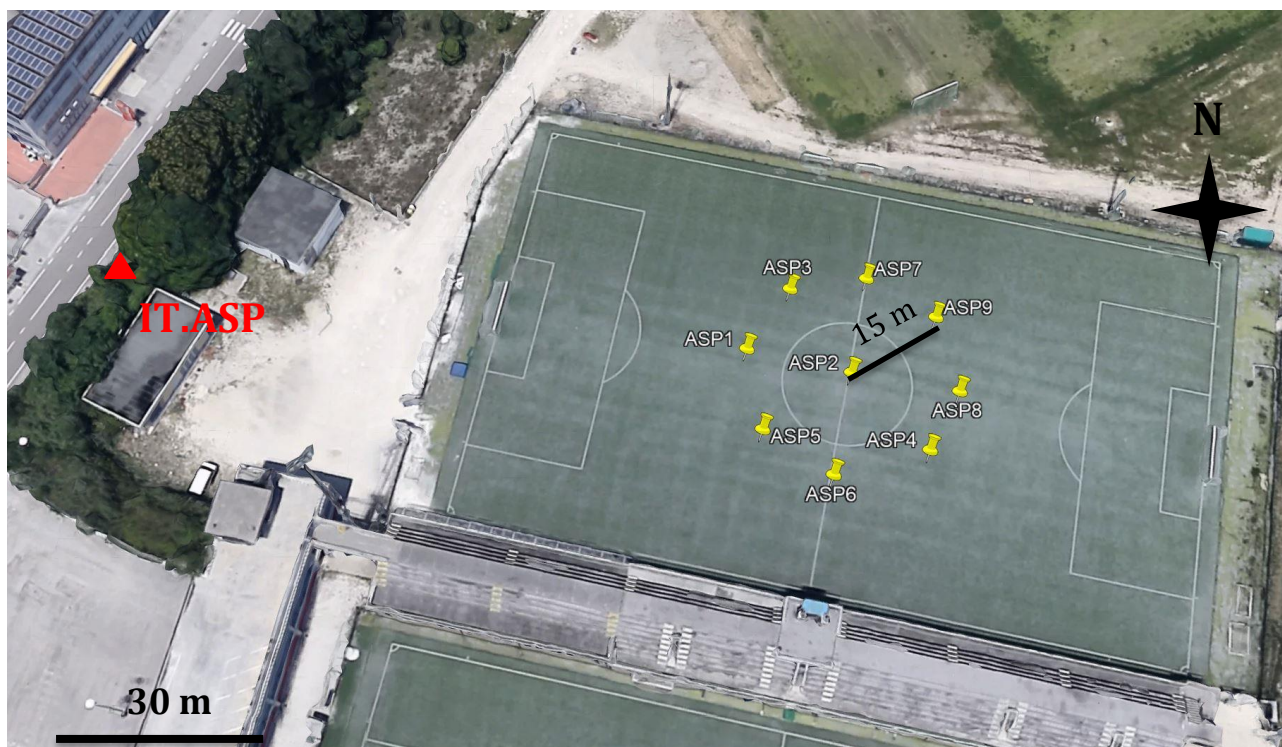
Figure 1: Map of the geophysical measurements performed at the IT.ASP site. The yellow points are the nine stations of the 2D array in passive configuration (all stations are equipped with Reftek-130 digitizer and Lennartz 3D-5sec velocimetric sensors). The red triangle indicates station IT.ASP.
