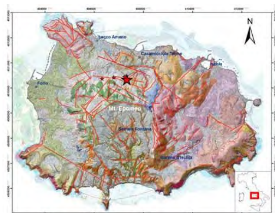
Figure 1: Faults (in red) are from Acocella and Funicello (1999), de Vita et al. (2010), Vezzoli (1988), Tibaldi & Vezzoli (1998) and geomorphological lineaments from Nappi et al. (2010). The base map is Carta Geologica dell'Isola d'Ischia della Regione Campania in scala 1:10.000, Foglio 464, 2011. The greatest red star is the 21 August 2017 main shock with the main aftershocks.
