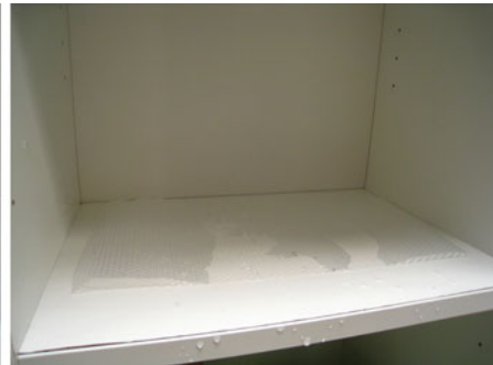
Fig. 23.6 Non-slip rubber mats can prevent movement of objects, but these should be used in dry surfaces. During the shake table tests, the fish bowl fell down due to the presence of water. Use of double-sided adhesive take is advised to secure fish bowls
