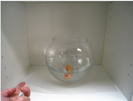
Fig. 23.6 Non-slip rubber mats can prevent movement of objects, but these should be used in dry surfaces. During the shake table tests, the fish bowl fell down due to the presence of water. Use of double-sided adhesive take is advised to secure fish bowls
