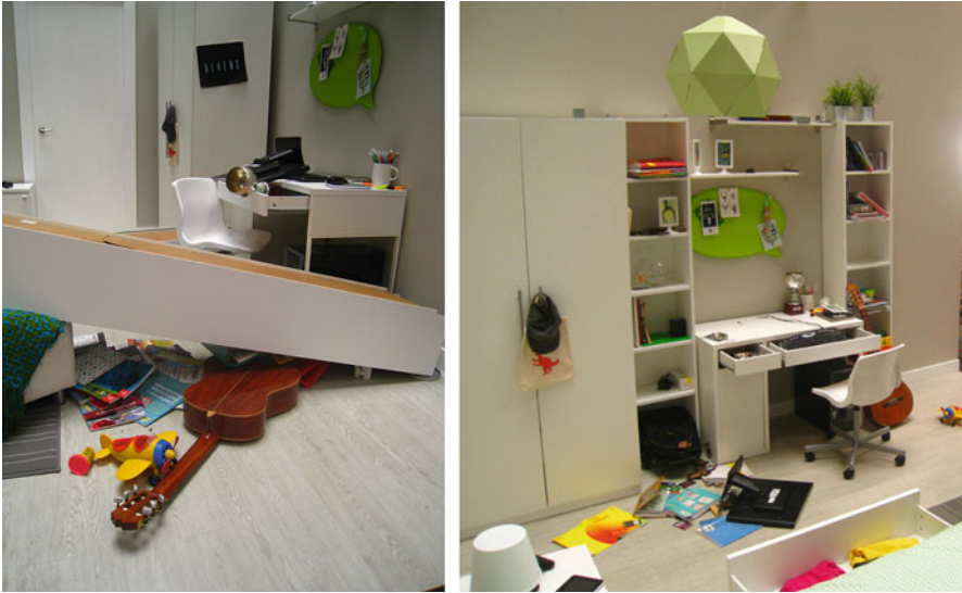
Fig. 23.9 Condition of unsecured (left) and secured (right) after shaking table tests
