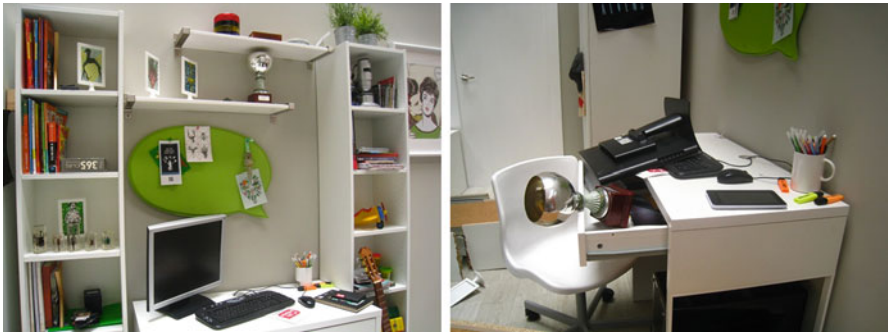
Fig. 23.3 Left: prior the shaking table test with unsecured objects. Right: after the shaking table test
