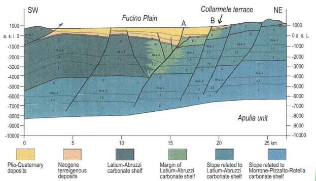
Fig. 10 - Geologic cross section of the Fucino basin interpreted from seismic reflection profiles. **A)** and **B)** locate respectively the San Benedetto-Gioia dei Marsi and Cerchio-Pescina-Parasano faults. Modified after Cavinato et al. (2002).
