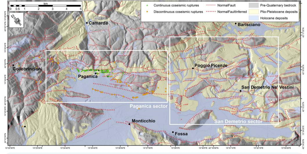
Fig. 16 – Map of the Paganica-San Demetrio Fault System (PSDFS) showing its geometrical arrangement at the surface and the extent and age of outcropping pre-Quaternary basement, and Plio-Pleistocene and Holocene deposits (modified after Civico et al., 2015).
