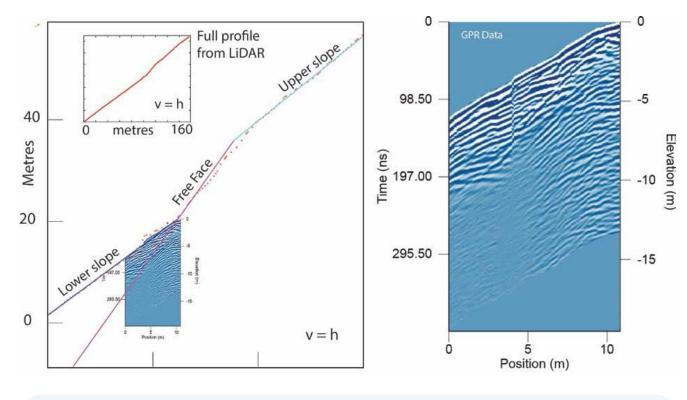
Fig. 34 - Scarp profile of the Serrone scarp from terrestrial LiDAR data, showing the classic geomorphology of upper slope, free-face and lower slope developed during the transition from cold to warmer climate across the demise of the Last Glacial Maximum (LGM). GPR data show the geometry of strata in the sub-surface, confirmed by exhumation of a trench.
